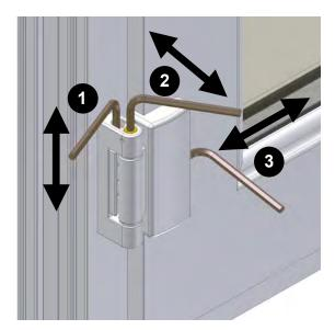
Vertical adjustment of each sash can be achieved by inserting the 5mm Allen key into
