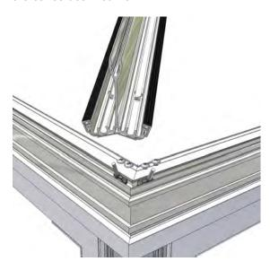
From the underside of the gazebo boss (C9026) pass a double bolt retainer (C9144) through the corresponding holes in the boss and the Victorian hip bar. (Please note that M5 x 20mm roofing bolts (C8017) may have been provided as an alternative fixing).
