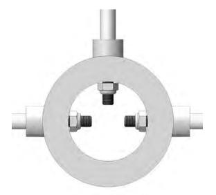
When all tie bar poles are in position and connected to all pole connectors, glazing bar lugs and ridge connection, you can now tighten the M10 tie bar centre boss locking nuts fully ensuring that the horizontal tie bar poles are tight fitting.
