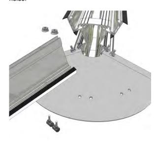
Slot the top of the Georgian hip bar over the double bolt retainer and loosely attach the M5 flange nut, but do not fully tighten at this stage. Repeat for the Georgian hips on the opposite ridge wing.
