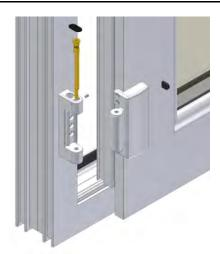
Once in position, pass the hinge pins through both hinge parts. It may be necessary to tap each pin down using a mallet. Do not fit the outer hinge cover and sash hinge cover caps at this time as some adjustment may be required later.
