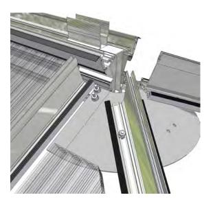
Push the roof glazing sheet up into the universal ridge wings then slowly allow it to slide back down away from the ridge until it rests flush with the bottom of the transom glazing bars.
