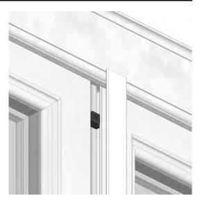
Fit the handles to all opening sashes using the 5 x 45mm handle screw (SC035).
