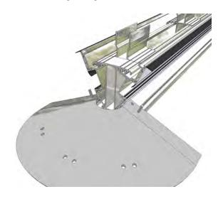
Once the boss end (C9170) is in position, locate the separate bolt through the predrilled hole in the underside of the universal ridge wing ensuring that the bolt passes through the hole in the boss end.
