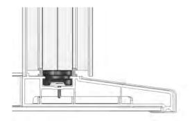
Position the window onto the 150mm sill (P106) and slide towards the first window.
