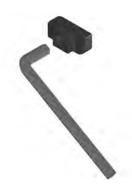
Position the quarter turn button (C105) longitudinally into the recess in the 90° corner post (A109).
