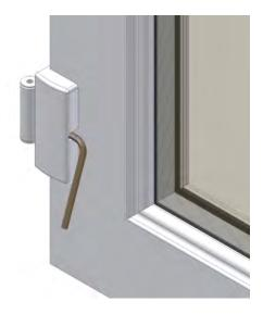
Horizontal (left to right) adjustment of the sash can be achieved by use of socket 3 located on the end face of the sash hinge cover (above). Insert the 5mm Allen key into the socket of the hinge and turn clockwise to move the sash inwards or anti-clockwise to move the sash outwards, Approximately 4mm adjustment can be obtained in either direction.
