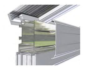
Select the eaves beam 135° joint cover (C9111), and push home into the corner gaps between the eaves beam internal cover (P6042).
