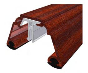
When the glazing bar top cap is attached, ensure that the bottom face of the top cap is aligned with the bottom face of the glazing bar. Remove the protective film from the glazing bar top cap.
