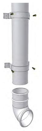
Connect the downpipe shoe (C9013) to the base of the downpipe. Fix the downpipe in position by use of the downpipe retention clips (C8056). They can be clipped over the downpipe and fixed into position with the screws provided
