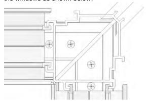
The prongs on the 90° corner post (A109) should face the outer corner of the 90° sill connector (C108) as shown below.
