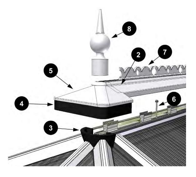
Now that all the edges of the polycarbonate roof sheets are sealed by use of the glazing bar top caps and the glazing bar end caps, the tops of the glazing bars need to be sealed from water ingress and dirt.
