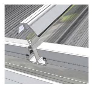
Use a glazing mallet or similar plastic surfaced mallet to knock on the glazing bar top caps starting at the top and working down the glazing bar towards the eaves beam (A5080).
