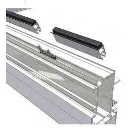
It is recommended to apply a bead of silicone to the gap between the eaves beam closure (P6056) and the glazing bar undercladding as shown below.
