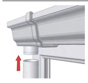
Push fit the downpipe (P6022) onto the spigot of the stop end outlet.
