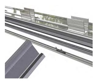
Repeat for the holes at the bottom of the transom glazing bars which connect to the M5 x 25mm bolts in the double bolt retainers located in the eaves beam. Loosely thread on the M5 flange nuts. Do not tighten at this stage.
