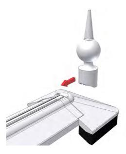
Slide the finial (C7012) fully onto the ridge capping as far as it will go.
