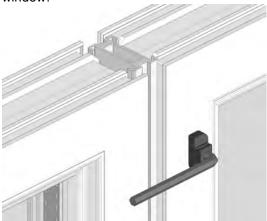
When the quarter turn button (C105) is in position and resting against the 18mm inline coupling (A104), turn the 6mm Allen key (CON046) 90° clockwise. The quarter turn button (C105) will 'click' into position.
