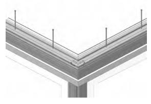
Do not use the 6.0 x 120mm yellow screws to fix the eaves beam (A5080) to the double door outer frame.
