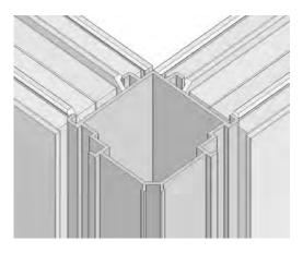
On Octagonal Garden Building models the 135° corner post (A115) is used. This should be assembled as shown below.
