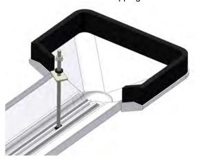
The ridge holding down bolts must be slotted into the groove on the underneath of the external ridge capping at approximately 500mm centres.
