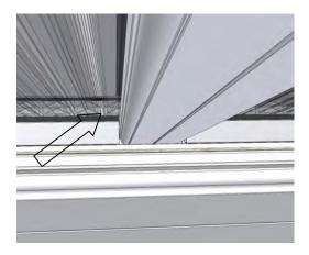
Select the eaves beam internal cover (P6042), position onto the barbs on the eaves beam (A5080) and press home.
