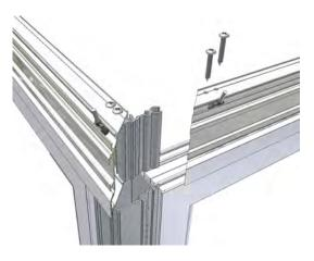
When all the eaves beams (A5080) are assembled on top of the windows, drill through the eaves beam only with a long reach 6mm drill at positions which are 100mm from the edge of each window (i.e. two holes per window position).
