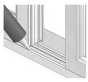
The window is slid along the 150mm sill (P106) until it is approximately 18mm away from the first window to be installed.
