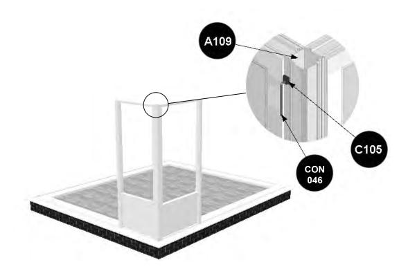
Select the first window to be installed. It is imperative that the drain slots in every window are located at the bottom of the window and facing front as shown below.
