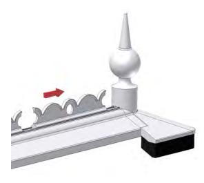
The last piece of cresting may have to be trimmed so that it finishes flush against the other finial when it is pushed onto the external ridge capping at the other end.
