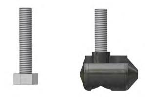
Slide a single bolt retainer into both of the universal ridge wings.
