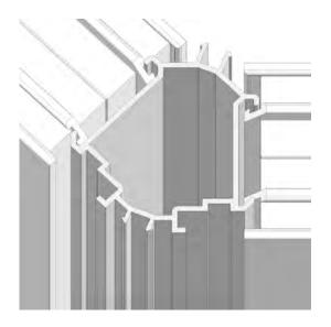
When the 90° corner post (A109) or the 135° corner post (A115) is in position, select a quarter turn button (C105) and the 6mm Allen key (CON046).
