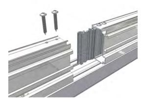
When in position, the eaves beam inline joiner (C9068) is fixed using the 6.35~x 38mm silver screws (C9132) through the pre-drilled holes.
