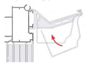
Where there are stop ends or outlets on the gutter you will need gutter joint clips to fix these in place. Offer the gutter joint clips over the gutter, slide up the back of the gutter until the hooks engages over the gutter. Pull up the front of the joints and clip over the gutter.
