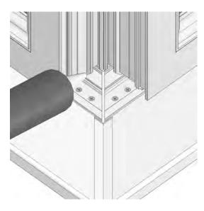
Select the 90° corner post (A109) and slide into the gap between the windows so that the leg detail interlocks with the leg detail on the windows as shown below.
