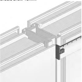
An application of silicone should be made to the 150mm sill (P106) where the 18mm inline coupling (A104) has made contact.
