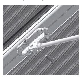
With the vertical tie bar rod and the two horizontal tie bar rods in place, raise them all together towards the centre and thread the ends of the tie bar rods through the holes in the 3 way tie bar centre boss.
