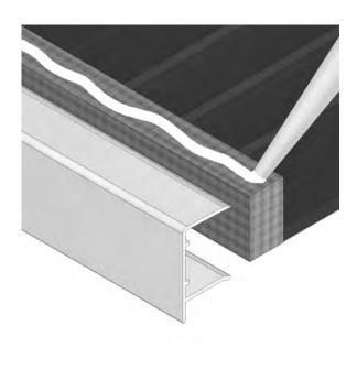
The glazing end trim push fits over the bottom edge of the roof glazing sheet with the flange facing downwards as shown below.
