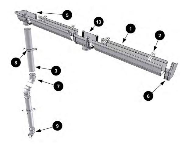
The following illustrations show the round downpipe located to the left hand side of the conservatory. This can however be fitted to either side. All the relevant components are supplied with your conservatory to suit either side.
