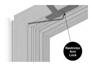
When the restrictor has been located, tighten the restrictor arm lock by using the 2mm Allen key.
