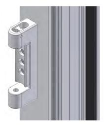
To hang the door, lift and slide the door sash assembly to allow the sash hinge adjuster to slide in between the outer frame hinge.
