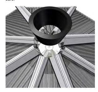
Once in position, seal the glazing and the hip and glazing bar top caps to the gazebo foam bung with a continuous bead of silicone.
