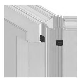
The 18mm coupling covers (P125) will require trimming to fit underneath the external eaves beam trim (P6024) and the eaves beam covers (P6042).
