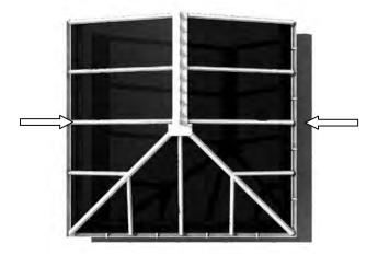
The lugs will be attached to the bottom of the relevant glazing bars where the tie bar is to be positioned. Three lengths of threaded tie bar rod and three lengths of conduit to cover the rod are supplied with each 3 way tie bar.
