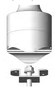
If you had to remove the bracket to insert the flange nut, re-attach the finial fixing bracket to the underside of the finial with the 4.0 x 25mm screws.
