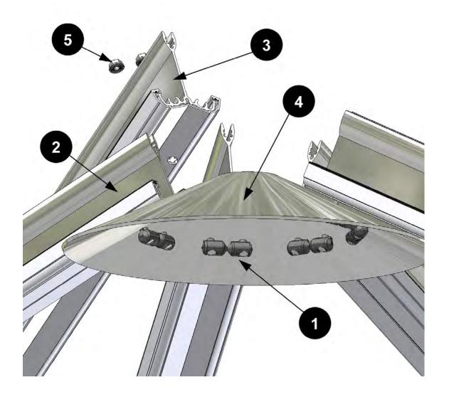
It will be easier to assemble the transom and Victorian hip bars if all the M5 flange nuts are removed from the double bolt retainers (C9144) in the eaves beam (A5080) and kept about your person for use as and when you require them.
