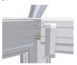
Prior to installing the square internal boss cover, it may need to be trimmed to the correct pitch of the roof
