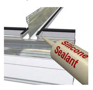
Although the glazing end trims (P6054) may already be fitted on the polycarbonate glazing sheets, they will have to be removed to allow the application a bead of silicone along the top face of the breather tape where it will come into contact with the glazing end trim. Re-attach the end trim once application is complete.
