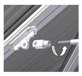
Once the rod has been attached to the clevis, the clevis can be fixed to the lug by means of the M10 nut and bolt. Attach both tie bar rods on the left and right sides of the conservatory in this way.
