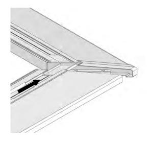
Note: Some sections may require joining by using in-line sill connector (C110).
