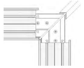
Silicone seal the internal corner of the 150mm sill (P106) where both windows meet.
