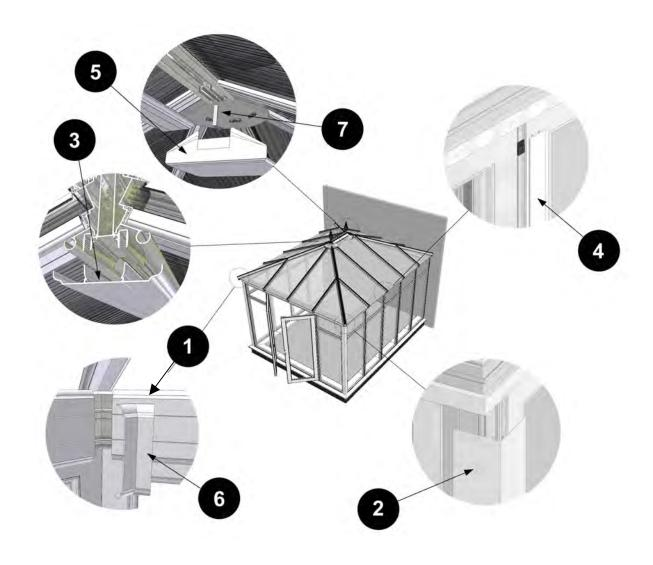
Check that you have sealed the joints in between the eaves beam closure (P6056) and the glazing bar undercladding on each window and that the glazing tape protective film has been removed.
