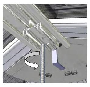
At this stage it is a good time to fit the ridge under cladding with the tie bar rod fitted in place. The ridge under cladding needs to be inserted and passed up the tie bar rod until it reaches the ridge centres and can be push fit onto the serrated prongs.
