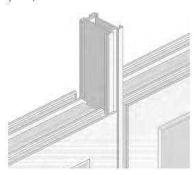
IMPORTANT: As the 18mm inline coupling (A104) is being positioned, check that the legs on the 18mm inline coupling (A104) interlock with the leg detail on the windows as shown at the top of the next column.
