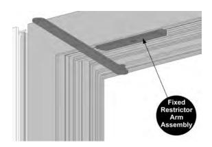
The restrictor arms are taped into position for transit. The tape should be removed prior to installation.
