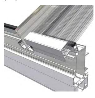
Allow the roof glazing sheet to gently rest on to the eaves beam closure (P6056).
