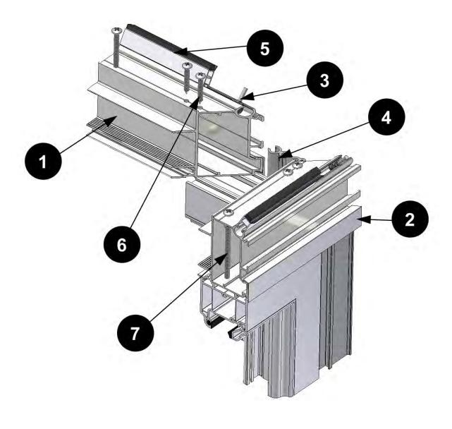
It is recommended at this point to re-check the internal window frame dimensions (width and projection) and check the measurements across the internal corners (these should be the same).
