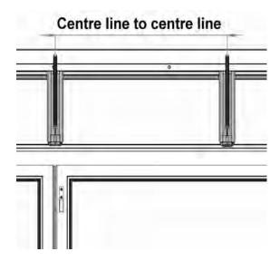
Now that all glazing bars are in position you must tighten all the M5 locking nuts which keep the glazing bars in place on the eaves beam.
