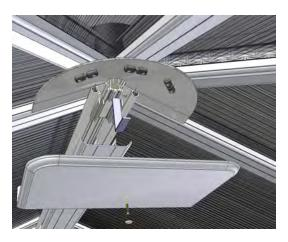
Select the ridge internal cover (P6042) and position beneath the serrated prongs of the aluminium ridge spacers. Push the internal ridge capping into position until it touches the bottom of the glazing bars on each side of the conservatory roof.
