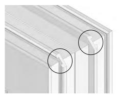
When the double door outer frame is in position on top of the 150mm sill (P106) the gap between the adjacent window and the door outer frame is approximately 18mm.
