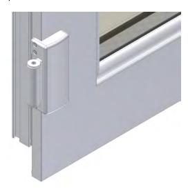
Two or three outer frame hinges and sash hinge adjusters are pre-fitted to the door outer frame. The hinge pin, hinge pin cover cap and hinge pin grub screw are supplied seperately.
