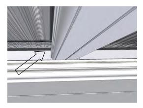
Select the eaves beam internal cover (P6042), position onto the barbs on the eaves beam (A5080) and press home.
