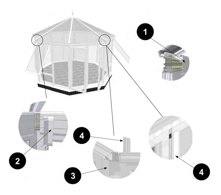
Check that you have sealed the joints inbetween the eaves beam closure (P6056) and the glazing bar under cladding on each window, and that the glazing tape protective film has been removed.
