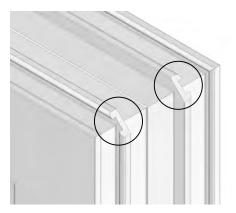
Select the first window and position over the milled out sections in the 150mm sill (P106).
