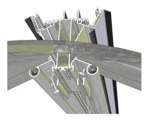
Permanently fix in place by use of a M5 flange nut.
