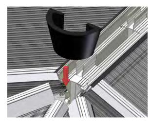
Using the silicone provided, run a continuous bead around the joint between the foam bung and the glazing and the glazing bar top caps, being careful to avoid gaps in the sealant.
