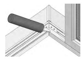
Continue to slide the window towards the corner of the sill so that the front edge is inline with the rear face of the 150mm sill (P106) on the adjacent corner.
