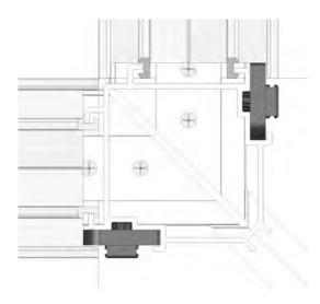
When both windows connected to the 90° corner post (A109) are in position, silicone seal the vertical joint between them to prevent water ingress. It is also recommended that you ensure the joint between the bottom edge of the window and the sill is also sealed.
