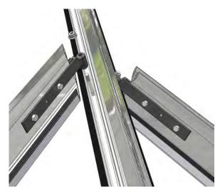
Slide the undercladding back to the top of the jack rafter and tight up against the Georgian hip undercladding. Locate the jack rafter onto the M5 x 25mm bolt in the eaves beam. Screw on the M5 locking nuts loosely. Do not tighten at this stage.
