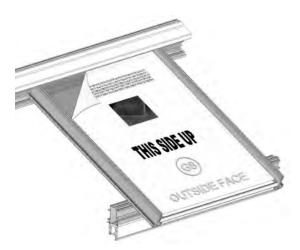
Prior to fitting the roof glazing sheets it is recommended to peel back around 50mm to 100mm of the glazing tape protective film. This enables adjustments to be made to the position of the roof glazing sheets without permanently sticking the entire roof glazing sheet to the eaves beam closure.
