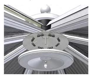
Locate the gazebo internal boss cover (C9032) over the nylon rod and secure in position by fully tightening the remaining flange nut.
