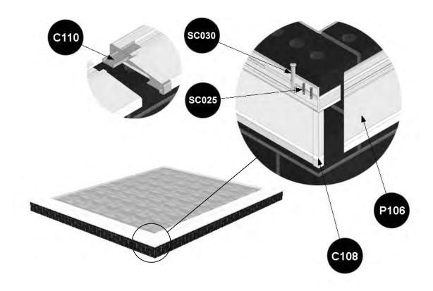
Having already inspected the base for LEVEL AND DIMENSIONAL ACCURACY (against base plan), lay out the 150mm sill pieces (P106) as per the conservatory plan.
