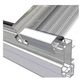
If positioned correctly there will be an approximate gap of 8mm between the sides of the roof glazing sheet and the centre stems on the jack rafters. The top edge of the roof glazing sheet will be approximately 5-10mm away from the centre stem on the Georgian hip bar.
