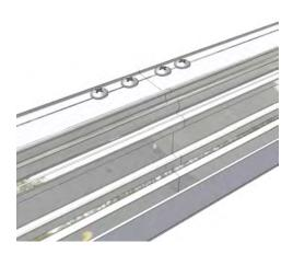
Attach the eaves beam external trim (P6024) onto the front of the eaves beam
