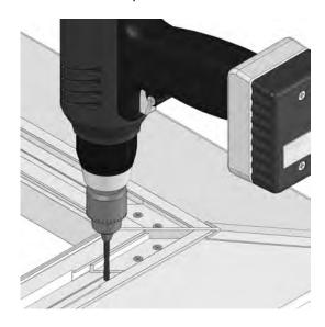
Now permanently fix through the 150mm sill (P106) to the base using the 100mm fixing bolts (SC030).
