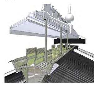
When assembling the external ridge cover, support can be gained by use of conservatory ladders or by spreading your leaning weight on boards positioned across the glazing bars. Do not put your weight directly on to the roof glazing sheets.
