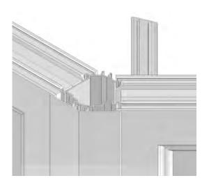
Select the 18mm coupling covers (P125) and position onto the recesses on the sides of each quarter turn button (C105) positioned on the 18mm inline couplings (A104) and press home.
