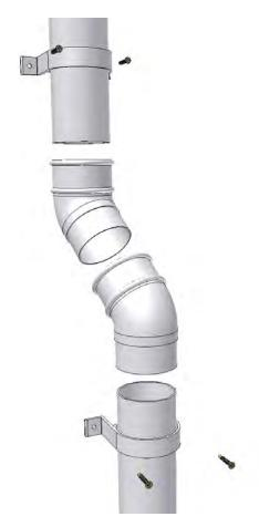
On dwarf wall models, you will need to cut the round downpipe (P6022) into two lengths and join them together by use of the downpipe bends (C9012). This is to allow the round downpipe to sweep over the 150mm sill (P106) and down the dwarf wall to the ground. The cut in the round downpipe is to produce two lengths that suit the height of the window frames and the dwarf wall.
