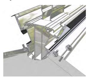
Start the ridge assembly by attaching the Georgian hip bars to the boss end (C9170). These are the glazing bars which run diagonally from the corners of the eaves beam (A5080) to the mini boss ends (C9170).
