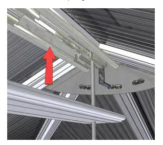
Thread the vertical tie bar conduit over the treaded bar and insert into the hole in the internal ridge cover. Leave the tie bar rod hanging down vertically from the ridge.
