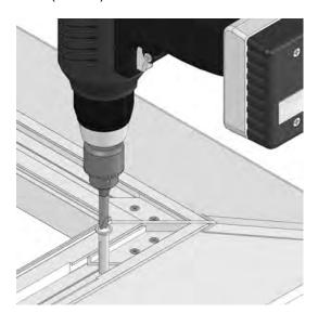
The 100mm fixing bolts (SC030) should be positioned 100mm from each end of the 150mm sill (P106) and equally spaced between.
