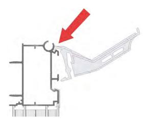
Pull the bracket downwards until it locks into place
