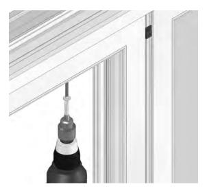
Silicone seal the gaps between the front of the eaves beam external trim (P6024) and the front of the windows to create a watertight seal.
