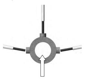
When the tie bar centre boss assembly is in place, thread on the M10 tie bar centre boss locking nuts. Check the horizontal tie bar rods for level before tightening the M10 tie bar centre boss locking nuts fully.
