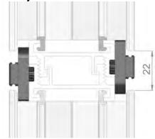
When the adjustable inline couplings (A107) are interlocked to the required setting they are slid between the two adjacent windows in the same way as the 18mm inline couplings (A104).
