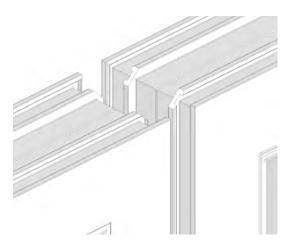
Take an 18mm inline coupling (A104) and slide it downwards into the gap between the two windows until it rests on the 150mm sill (P106) at the foot of the window.
