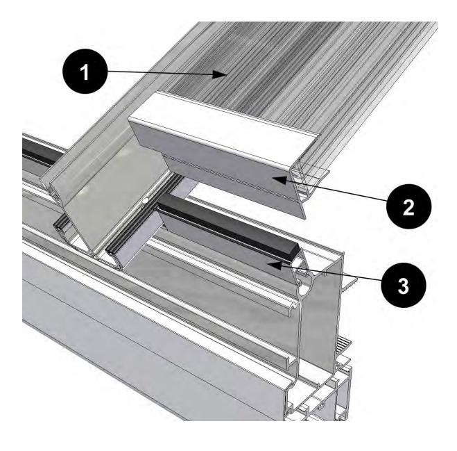
Unpack the roof glazing sheets. If your glazing material is polycarbonate, it is important at this stage to note that the surface which is protected by the *printed* polythene film is the surface that is on the outside of the conservatory. The print on the outer film gives details on how to correctly store your polycarbonate until it is installed. Each roof glazing sheet is labelled with the corresponding number on your roof plan.
