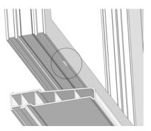
The windows are permanently fixed together in the same way as any other window using the quarter turn buttons (C105) and the 6mm Allen Key (CON046) as described previously.
