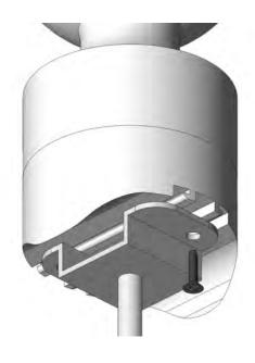
Drill a 10mm diameter hole through the centre of the Gazebo Boss (C9031) and insert the rubber grommet from the gazebo fixing kit (C9054) into the hole.
