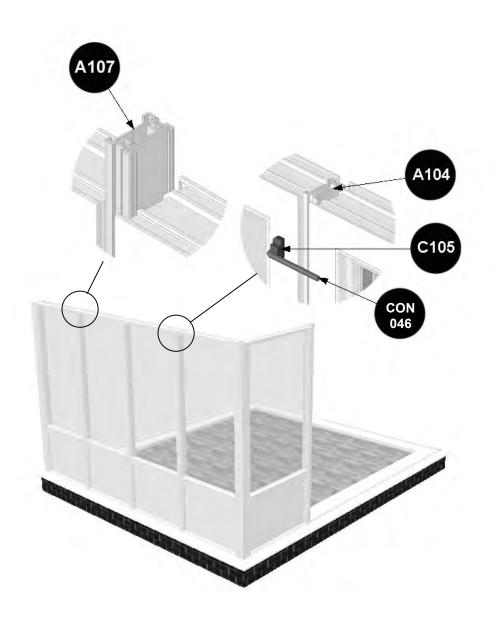
Select the window to fit against the previously installed window. It is imperative that the drain slots in every window are located at the bottom of the window and facing front as shown below.
