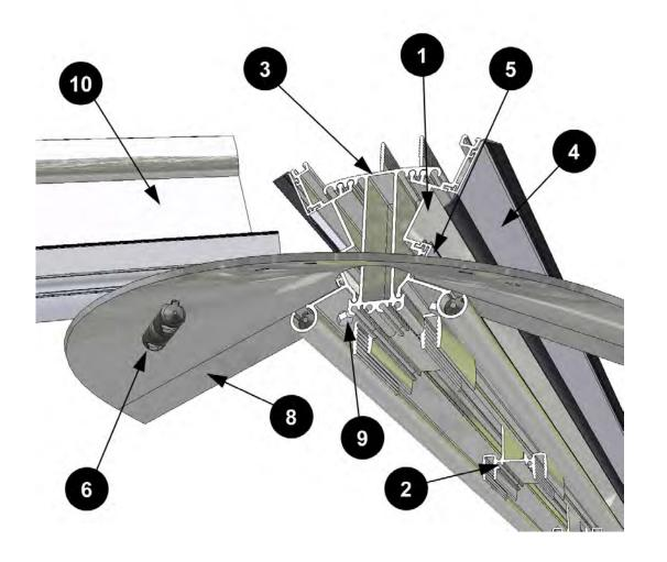
Referring to your roof plan, select the correct number of bolt retainers (C9144) complete with M5 x 25mm bolts (C9142) and slide into the channels of the universal ridge wings (A5081).
