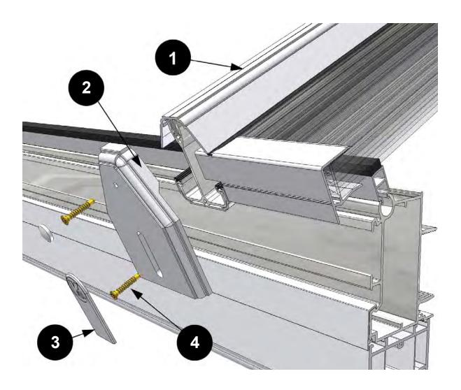
Once all roof glazing sheets are in position and stuck to the eaves beam closure, it is time to attach the top caps to the glazing bars. This is for two reasons; firstly to
