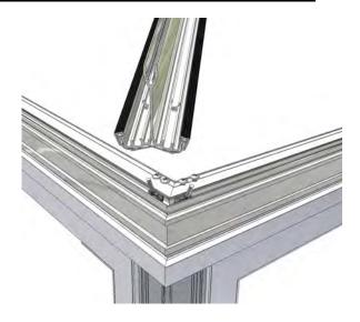
Now locate a double bolt retainer from underneath the boss end and through the holes.
